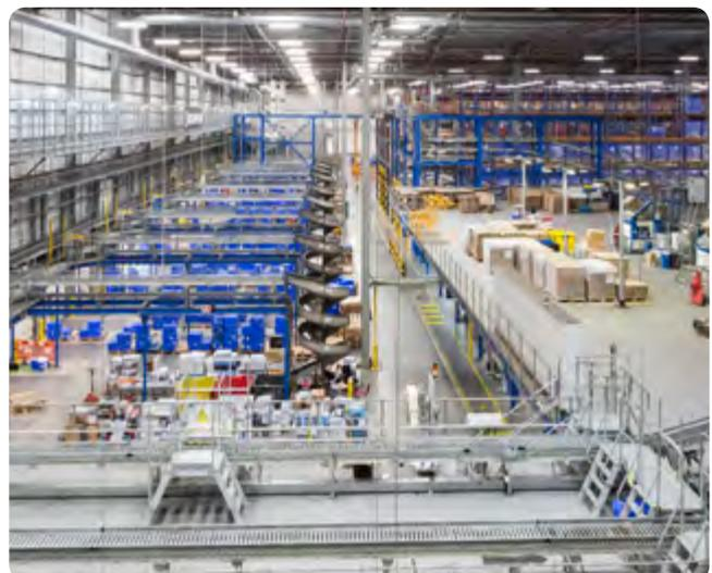
To drive efficiency, occupiers increasingly invest in advanced systems that allow them to stock automatically and rapidly retrieve products, so they can operate on a “just in time” basis.
